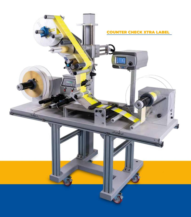
When working as a control device, a photocell counts the labels but is also able to check their presence and signal their absence with the possibility of stopping for repositioning. The operation doesn't require settings as it is performed by the control unit which acquires the label length by self learning. An ultrasonic photocell is available for transparent labels.
